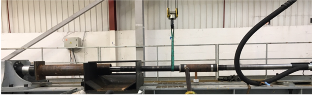
Drilling test set up on HydroVolve test rig
