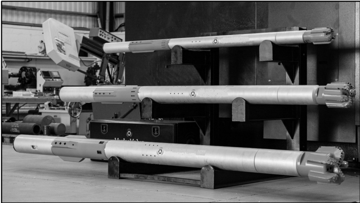
Figure 7: -The Complete System with PDC bits - 6" (top), 8-1/2" (middle), 12-1/4" (bottom)
