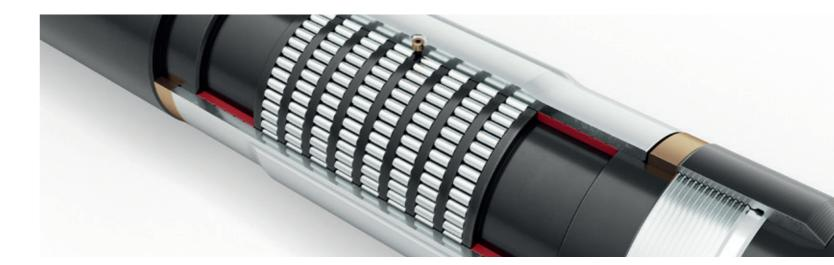
MonoVolve REDUCER is a drillstring sub which reliably reduces the effects of side-loading and high torque associated with rotation of the drill string in the cased and open hole. It's ultra-durable single-bodied, single-sleeved design has been developed specifically with rugged reliability at its core.
