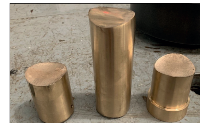
Double-pin shear test: 75,000klbf overpull, 360,000klbf impact shear
