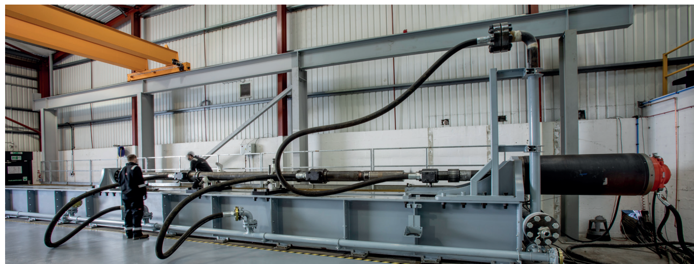
Testing at HydroVolve drilling test centre: 550Tonne (1,200,000lbf) push-pull test rig, 120RPM Drive @ 13.5kNm (10,000ft.lb) Torque, 350Bar (5000psi) Flow Loop.
