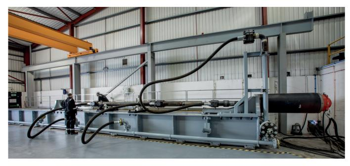
Testing at HydroVolve drilling test centre: 550Tonne (1,200,000lbf) push-pull test rig, 120RPM Drive @ 13.5kNm (10,000ft.lb) Torque, 350Bar (5000psi) Flow Loop.
