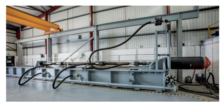
PolyVolve SWIVEL DS passed qualification testing for **maximum customer load** over a **24 hour rotating duration** at **60RPM** in both **tensile and compressive load** modes **with no damage** or loss or performance.
